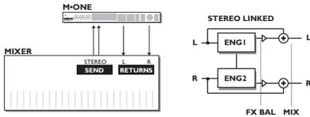
In the Stereo Linked Routing the Engines perform the exact same effect with synchronized parameter settings. Left I/O are used for Engine 1, Right I/O are used for Engine 2. When switching to Stereo Linked Routing the Engine 1 settings are forced into Engine 2.
