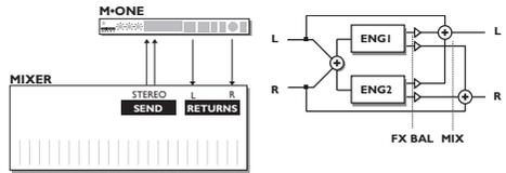
The Parallel routing sums left/right Inputs, and both Engines are fed with the exact same signal. As illustrated the unprocessed dry signal is mixed with the processed signal into two channels via the Mix parameter.
