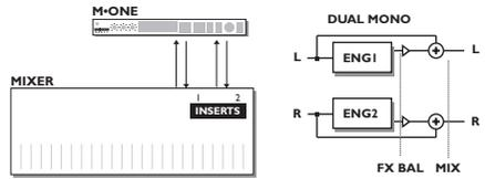
In the Dual Mono routing, the two Engines are totally independent, meaning mono in/mono out of each Engine. Left I/O are used for Engine 1, Right I/O are used for Engine 2.
