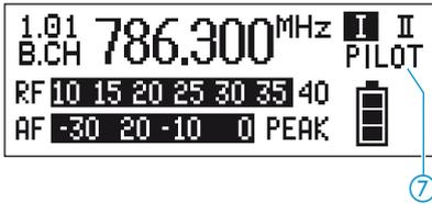
The “PILOT” display ⑦ appears on the display panel when the pilot tone evaluation is activated (see “Activating/deactivating the pilot tone evaluation” on page 25).
