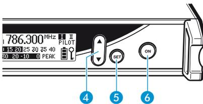
During standby operation, the ON button ⑥ is backlit in red. When the receiver is switched on, the SET button ⑤ and the ▲/▼ button ④ are additionally backlit in green.
