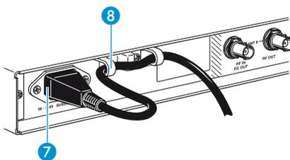
Use the mains cable to connect the twin receiver to the mains (90–264 V AC, 50–60 Hz).
