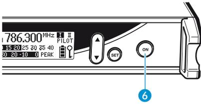
Each receiver of the EM 550 G2 is switched on and off separately with the **ON** button. The receivers can only be switched off when the standard display is shown on the display panel. When in the operating menu, briefly pressing the **ON** button will cancel your entry (ESC function) and return you to the standard display with the last stored settings.
