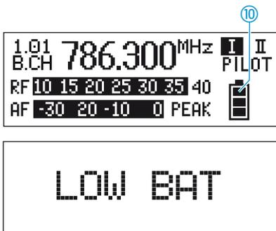
The 4-step transmitter battery status display ⑩ provides information on the remaining battery/accupack capacity of the received ew 500 G2 transmitter:
