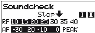
By doing a soundcheck, you can check the reception area for field strength gaps ("dropouts") which cannot be compensated for by the receiver's diversity circuitry. You can do the soundcheck without the help of another person.
